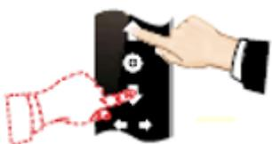
Press arrow "up" or "down" and hold until the motor reaches the desired position.
