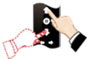
Press "arrow up" or "down" and adjust the desired limit position.
